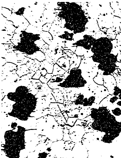
Alloy 46. Annealed at 1300°F. (704°C.) for 15 hours. Nitric acid etched. 105X.
